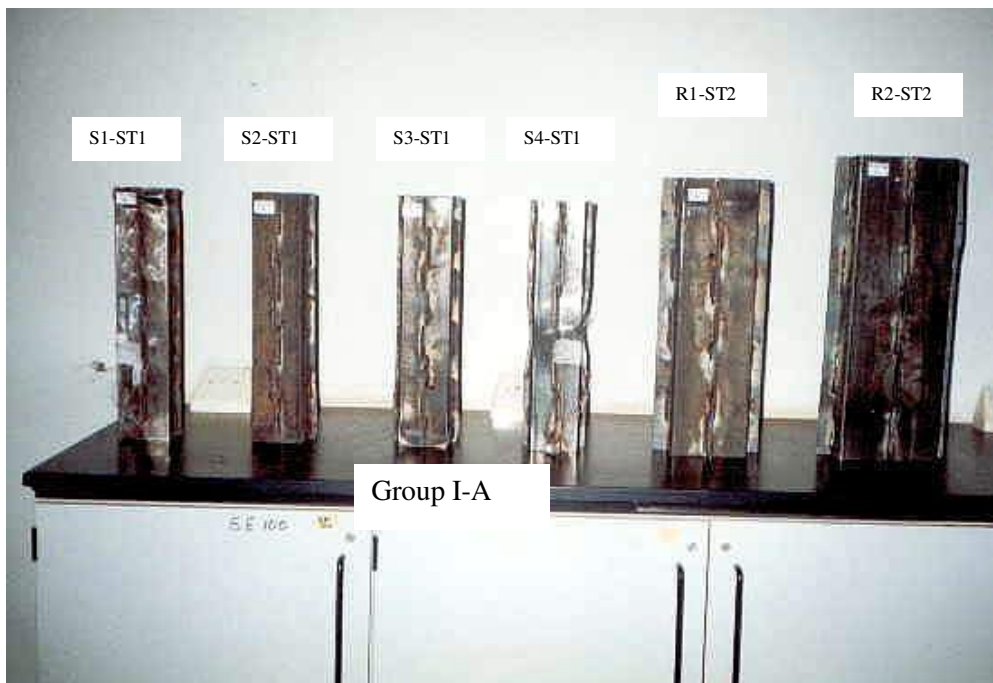
Fig.5.3 Stiffened tubes after failure, Group I-A.
