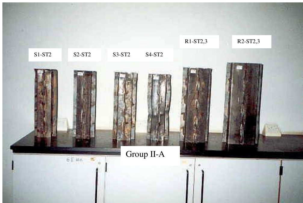
Fig.5.5 Stiffened tubes after failure, Group II-A.
