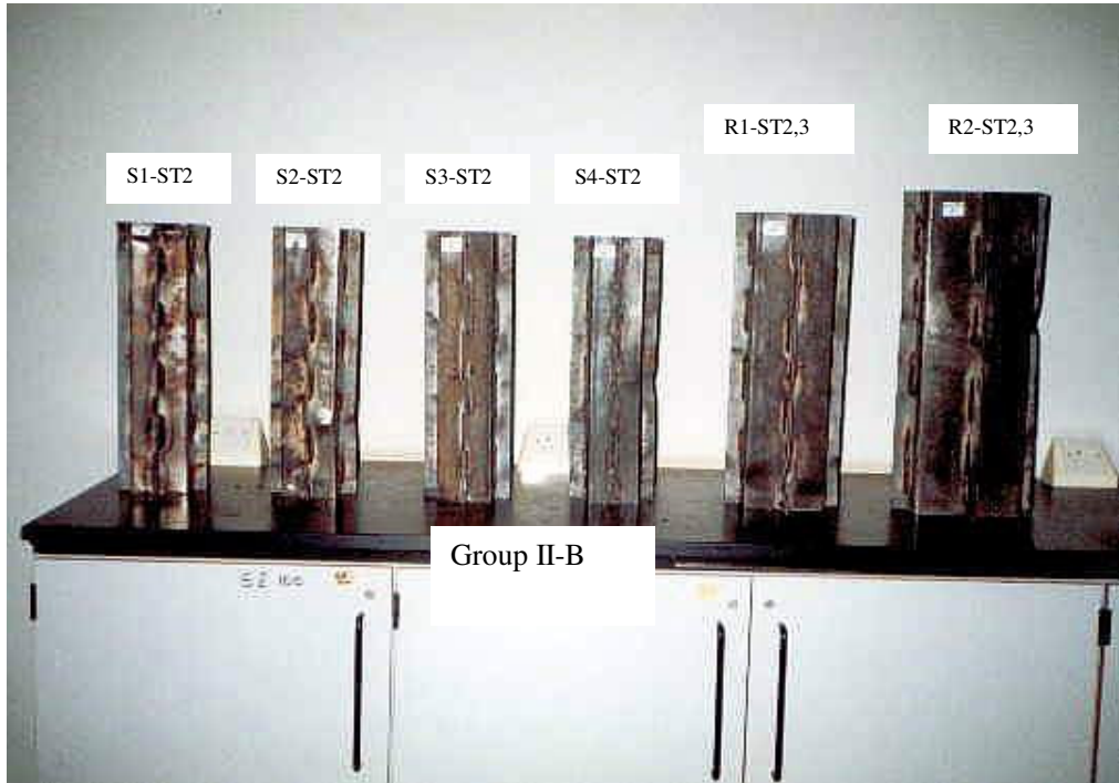
Fig.5.6 Stiffened tubes after failure, Group II-B.
