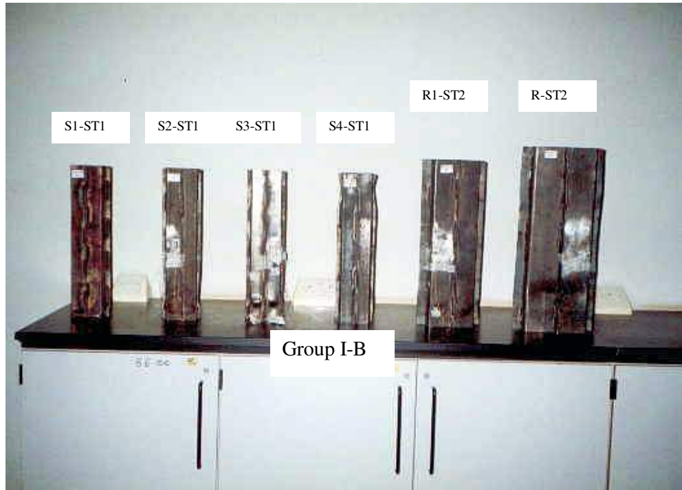
Fig.5.4 Stiffened tubes after failure, Group I-B.
